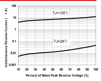
Fig.2-Typical Reverse Characteristics
