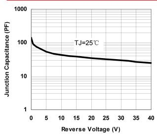
Fig.1-Typical Junction Capacitance
