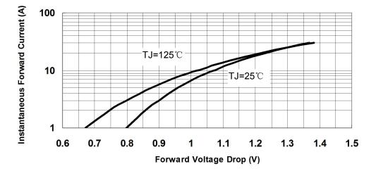
Fig.3-Typical Instantaneous Forward Voltage Characteristics
